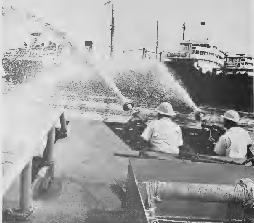
HUNDREDS OF gallons of foam shoot out of the turrets in a scene that resembles combat action aboard a naval vessel. Fire-fighters can handle the turrets with ease and direct foam or water with high accuracy.
